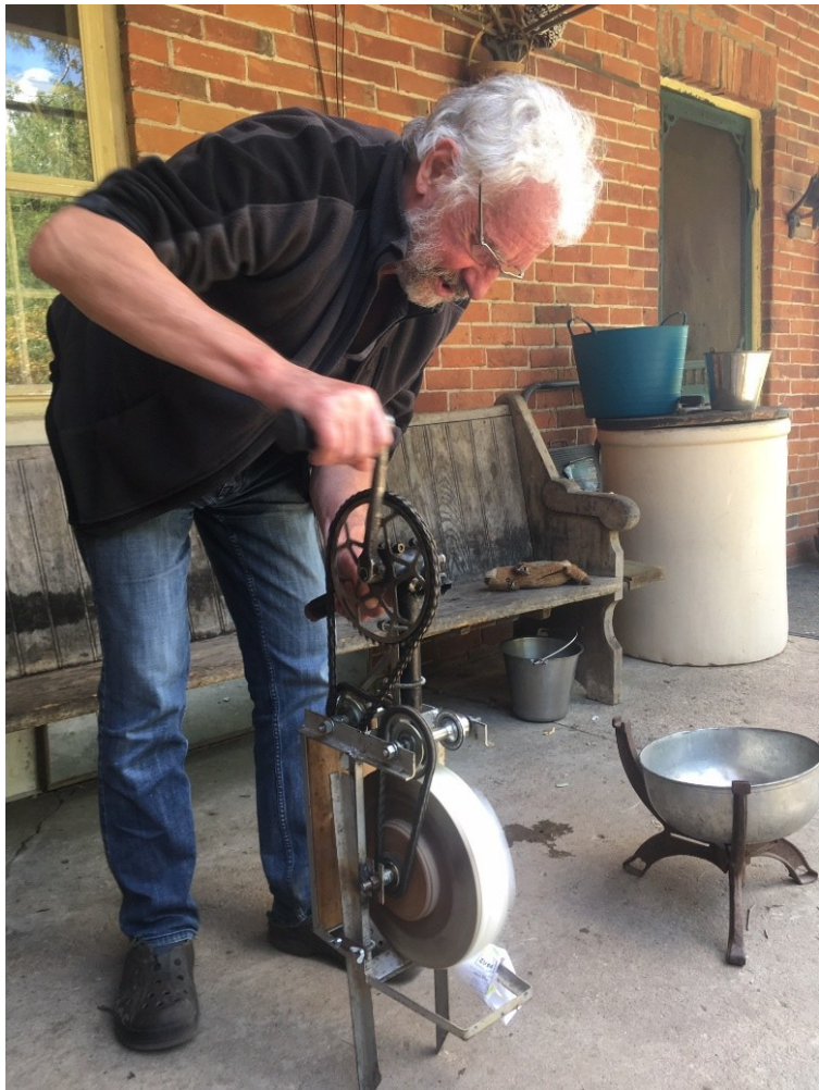
Richard Hawkins demonstrating a hand-driven lure machine originally designed for training (amateur) track Greyhounds in straight gallops
